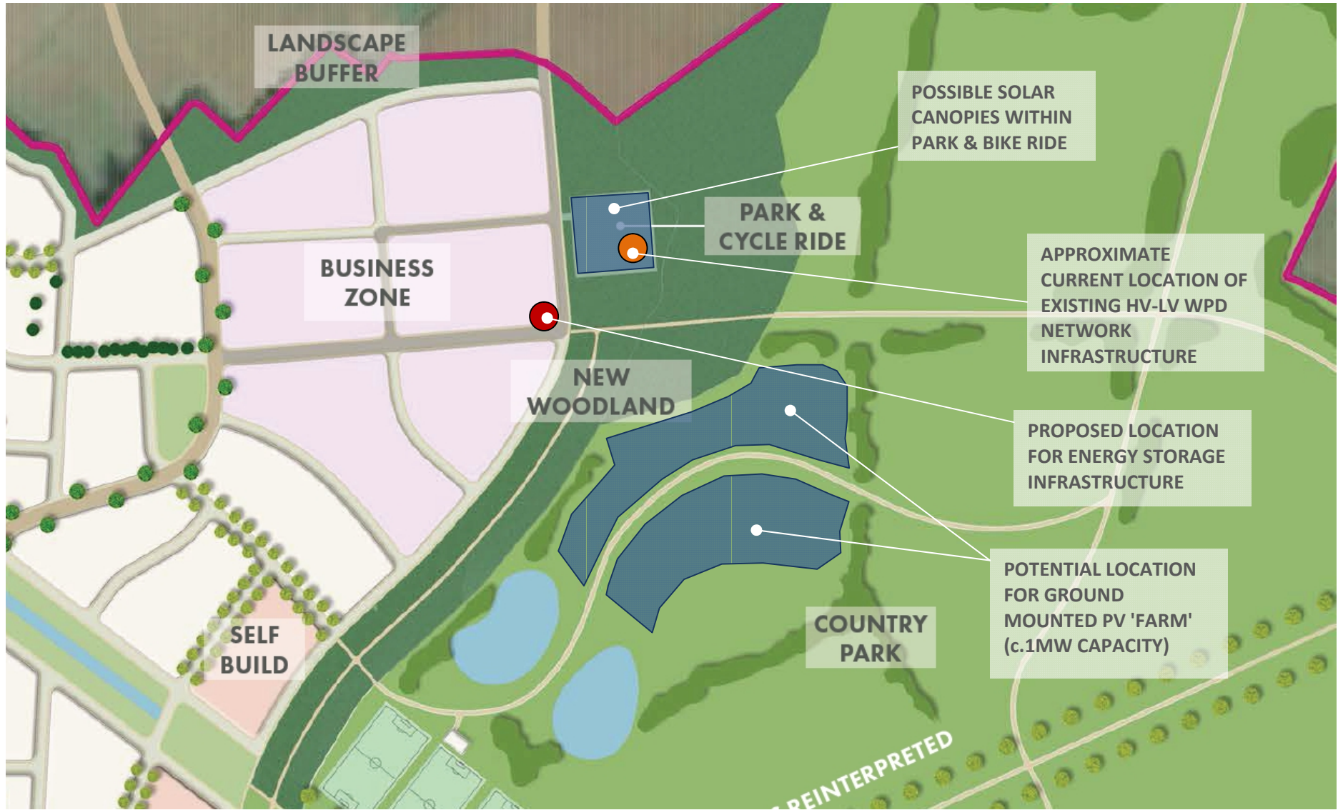
Figure 2: Additional PV and Energy Storage Locations
