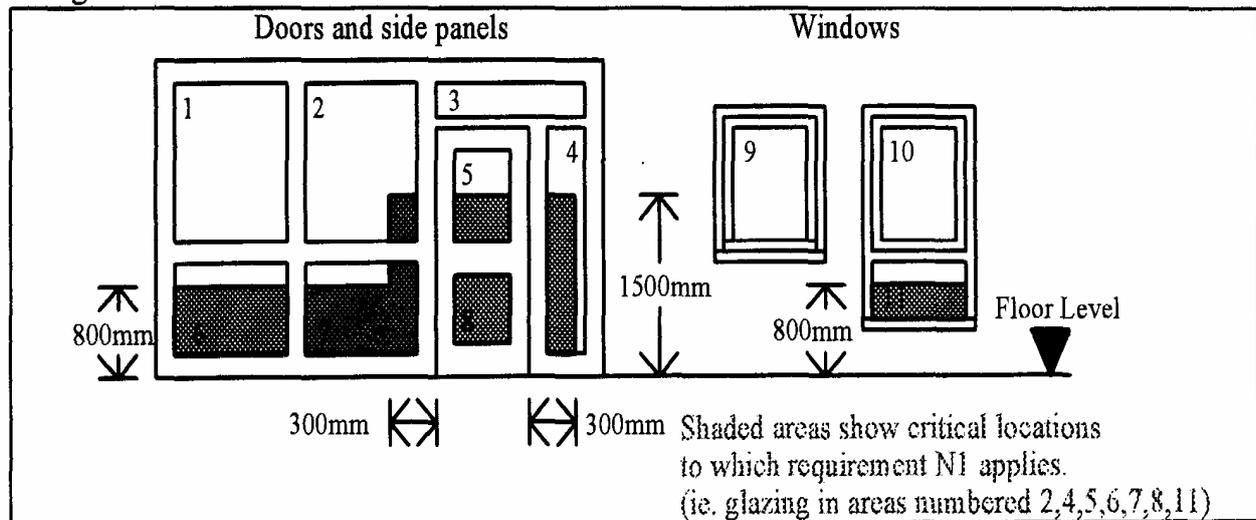
**Glazing in 'Critical Locations' should break safely**, i.e. laminated or toughened Class C safety glass complying with BS6206. Or if it is installed in a door or in a door side panel and has a pane exceeding 900mm it should be Class B of BS 6206.
